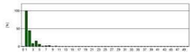
Figure 6 Unfiltered current harmonic spectrum
