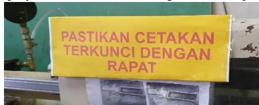
Figure 8. Mold Locking System Visual Display Implementation
