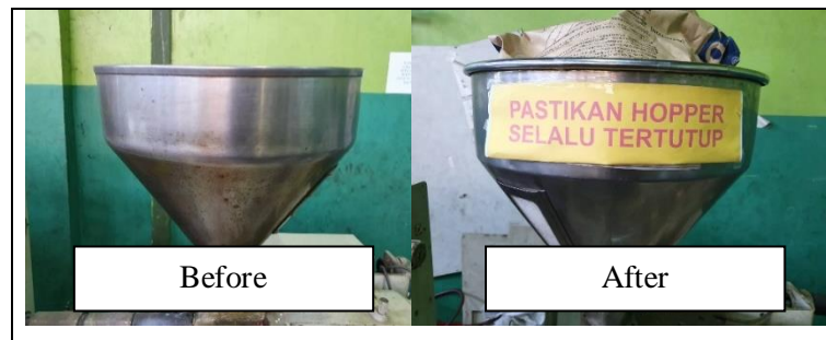
Figure 7. Hopper Closing Visual Display Implementation
