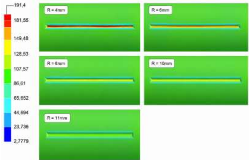
Figure 2 Von Mises stress distribution across the five repair-radius models (unified legend, 2.78–191.4 MPa)
