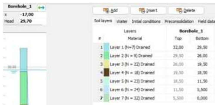
Figure 1. Soil layer on undrained 2D Plaxis Modeling
