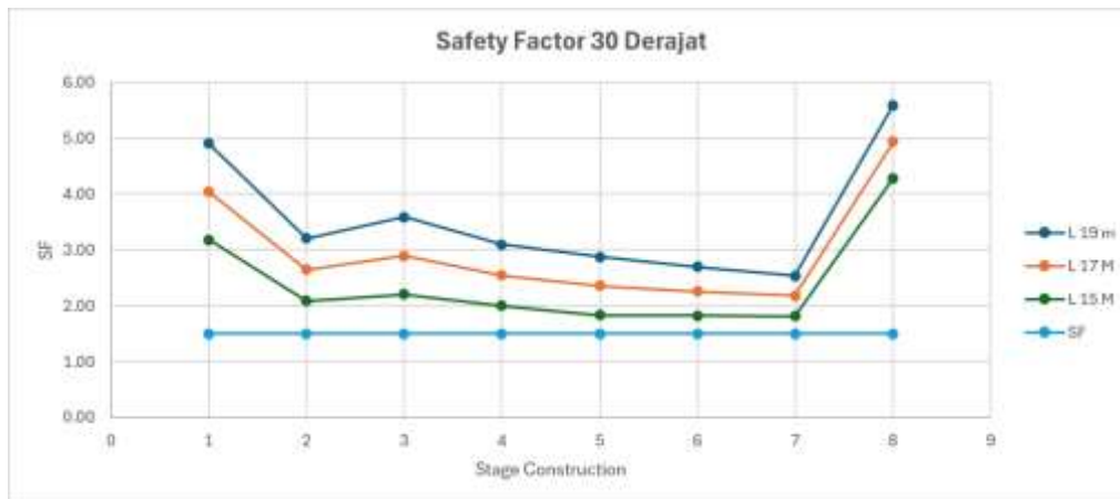
Figure 18. SF or FKpo Pseudostatic variation of 30o angle nails 19 m, 17 m and 15 m
