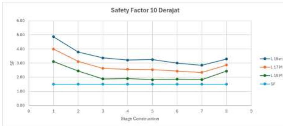
Figure 16. SF or FKpo pseudostatic variation of 10o angle nails 19 m, 17 m, and 15 m
