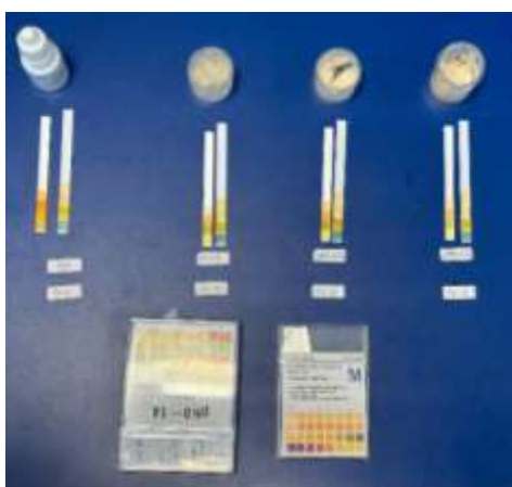
Figure 3 pH measurement of J. multifida Linn in multiple concentrations using universal pH paper.
