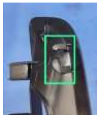
Figure 2. Defect Short shot Source: Documentation (2025)
