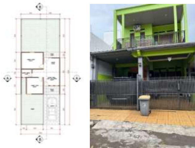
Figure 8. Floor Plan of the Original Type 41 House Before Expansion (Left) and a Type 41 House After Expansion (Right)
