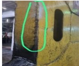
Figure 1. One Type of Failure: Crack on the Lifting Coil C – Hook Source: Documentation from PT. X
