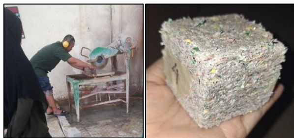
Figure 1. Surface Grinding Process and Cubic Test Specimen of Paving Block
