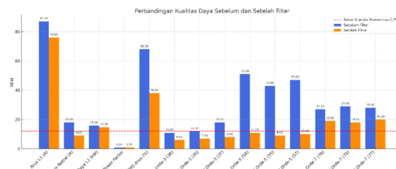
Chart 21. Power quality parameters and IHD before and after filter installation
