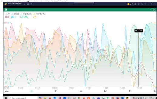
Figure 10. Trend graph of electrical parameters before filter installation
