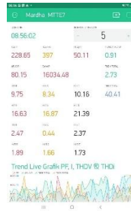
Figure 15. Blynk Monitoring Display After Installing the Harmonic Filter
