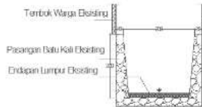
Figure 3. Existing Dimensions of Cassowary City Drainage Channels
