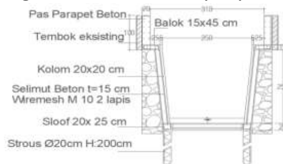
Figure 4. Recommended dimensions of Cassowary city drainage channels
