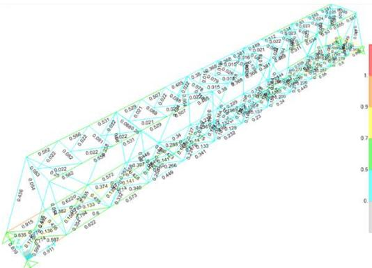
Figure 16. PMM Ratio (Dimensional Correction)
