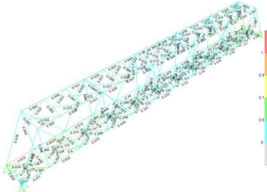
Figure 15. PMM Ratio (Dimensional Correction)
