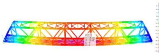
Figure 13. Bridge Deflection (Unit: mm)
