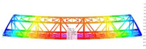
Figure 10. Bridge Deflection (Unit: mm)
