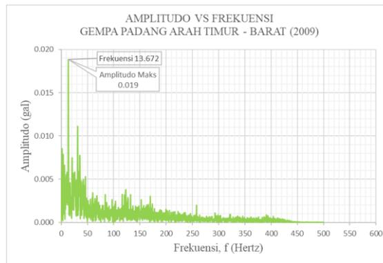
Figure 7. Earthquake Frequency (East-West)
