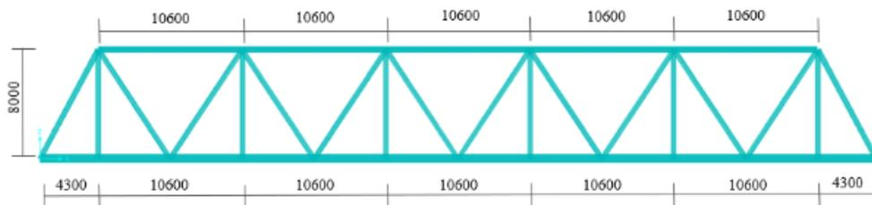
Figure 4. Side View of The Model
