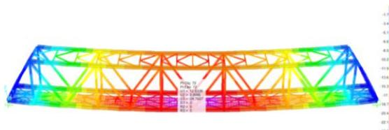
Figure 12. Bridge Deflection (Unit: mm)
