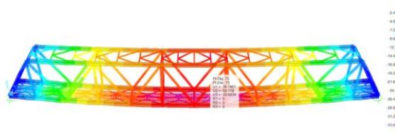
Figure 11. Bridge Deflection (Unit: mm)
