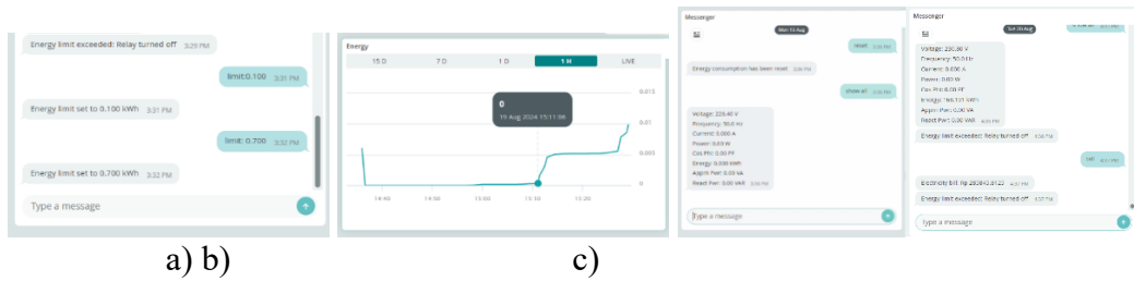
Figure 5. a) Set limits and automatic messages if consumption reaches the limit; b) Energy graph when reset; c) Display 8 parameters of sensor & bill measurement results
